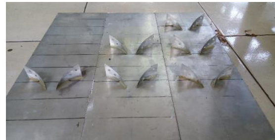
Fig. 5. CRWVGs test plate with 30°, 45°, and 60° angle of attack
