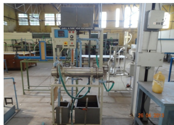
Fig.1 Experimental setup for Shell and Tube Heat Exchanger
