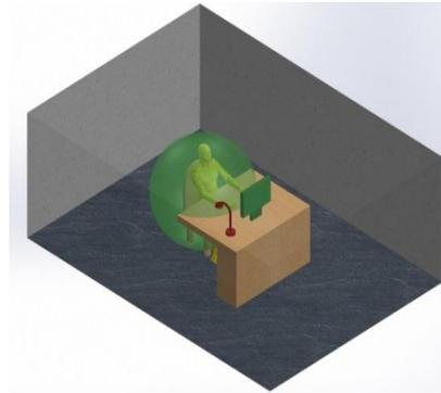
**Figure 1.** A schematic view of the desk displacement ventilation concept and the definition of micro/macro-climate area
