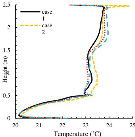
Figure 8. The temperature gradient in front of the occupant
