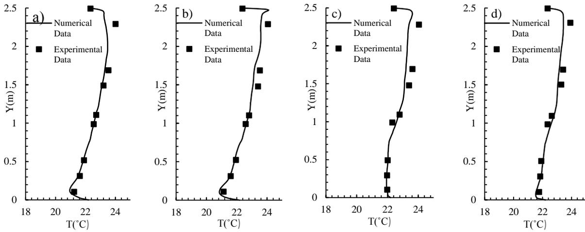
Figure 4. Comparison between CFD simulation and experimental data of temperature gradient along; (a)  $x=1.5\text{m}$  and  $z=0.68\text{m}$ , (b)  $x=1.5\text{m}$  and  $z=2.43\text{m}$ , (c)  $x=3.75\text{m}$  and  $z=1.93\text{m}$ , (d)  $x=3.75\text{m}$  and  $z=2.93\text{m}$
