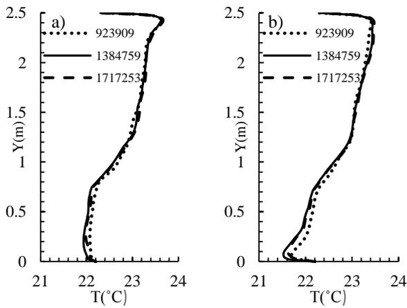
Figure 5. the grid independent test along; (a)  $x=3.75\text{m}$  and  $z=1.93\text{m}$ , (b)  $x=3.75\text{m}$  and  $z=2.93\text{m}$
