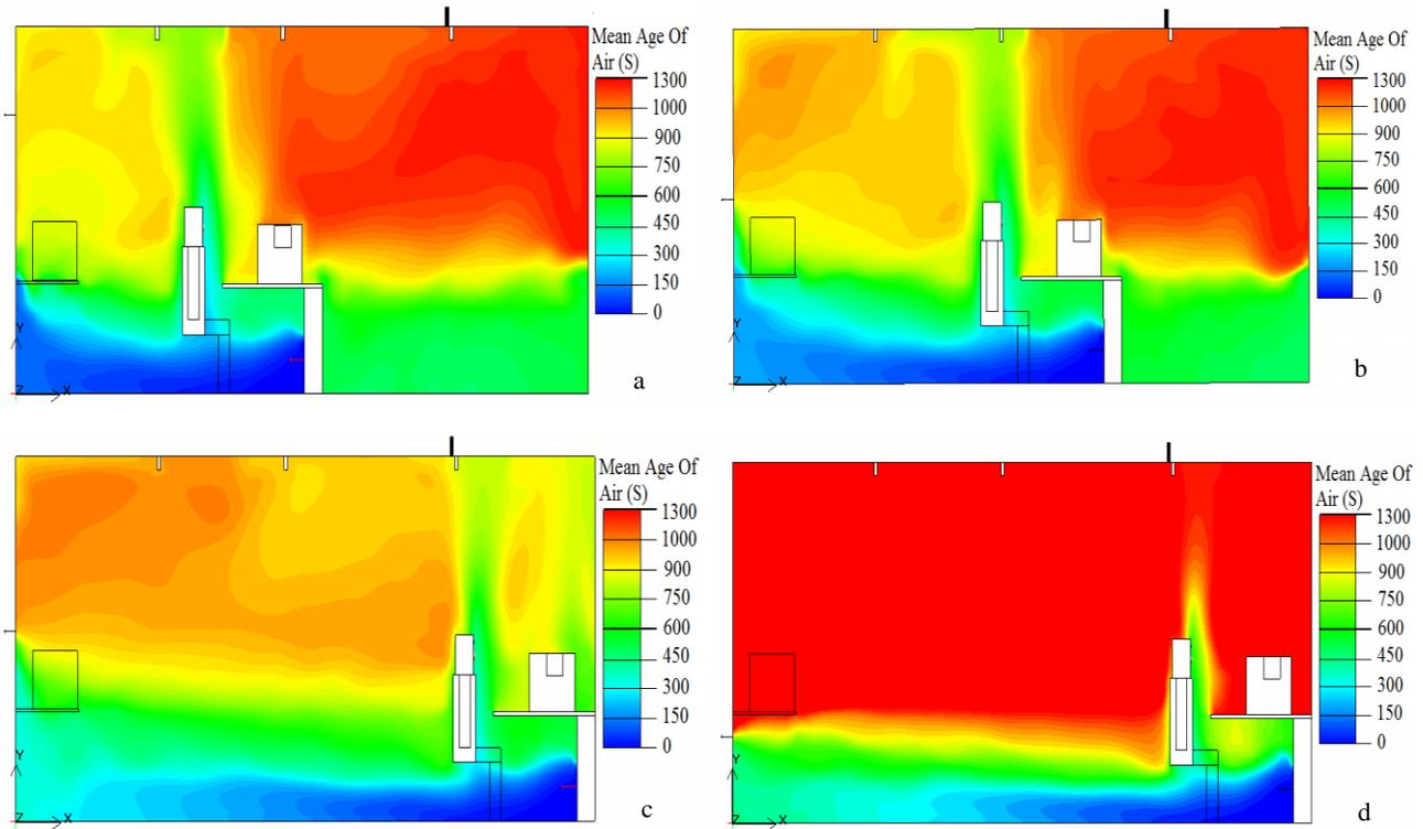
Figure 10. The Mean age of air of the room; (a) case 1, (b) case 2, (c) case 3, (d) case 4
