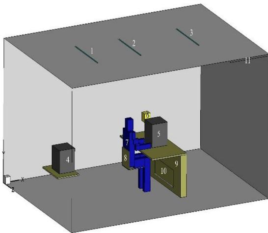
Figure 2. Configuration of the test chamber; 1-3 lamps, 4-5 Pc simulator, 6- light simulator 7- occupant, 8- chair, 9- supply unit, 10- displacement diffuser, 11- exhaust vent.
