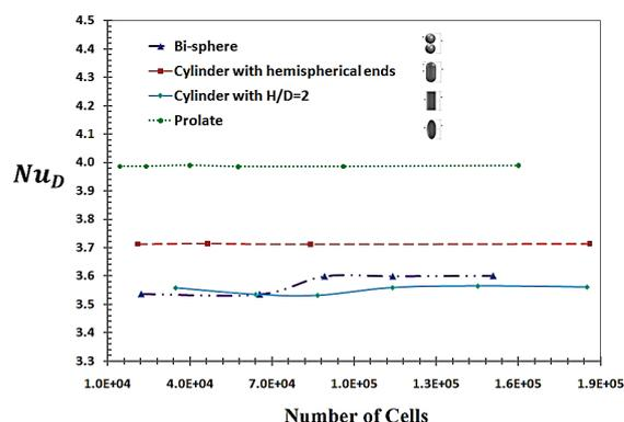
Figure 3. Effect of grid resolution on free convection heat transfer from at  $Ra_D = 1.76 \times 10^3$
