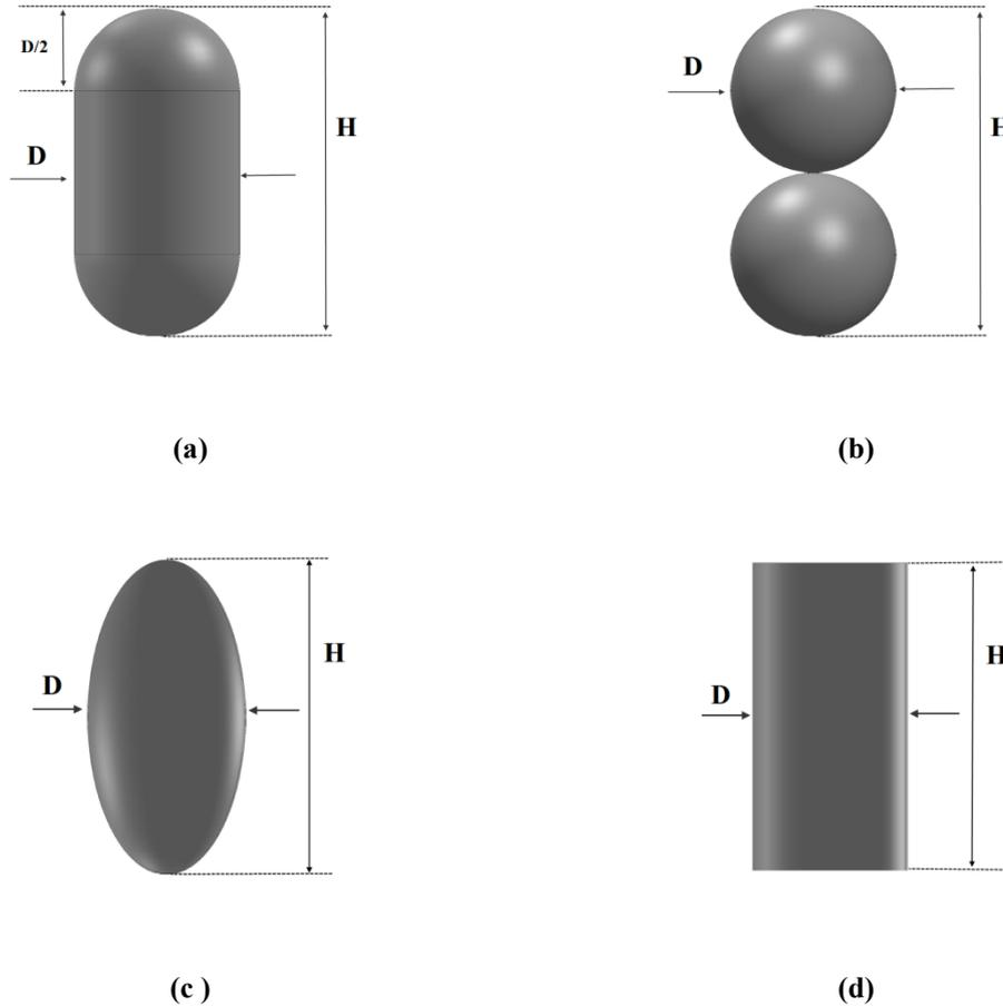
Figure 1. Geometry of different body shapes in the present study; a) Cylinder with hemispherical ends, b) Bi-sphere, c) Prolate, d) Cylinder
