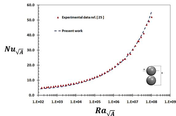
Figure 4. Comparison of the present numerical results for a bi-sphere with experimental data of Jafarpur [25]
