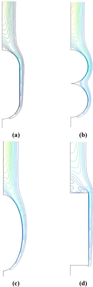
Figure 8. Streamlines near the bodies' surfaces; a) Cylinder with hemispherical ends, b) Bi-sphere, c)
