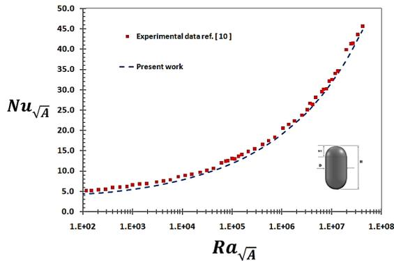
Figure 5. Comparison of the present numerical results for a cylinder with hemispherical ends with experimental data of Jafarpur [10]
