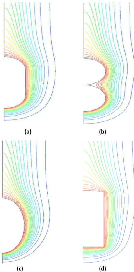
Figure 6. Isothermal contours around the bodies' surfaces; a) Cylinder with hemispherical ends, b) Bi-sphere, c) Prolate, d) Cylinder
