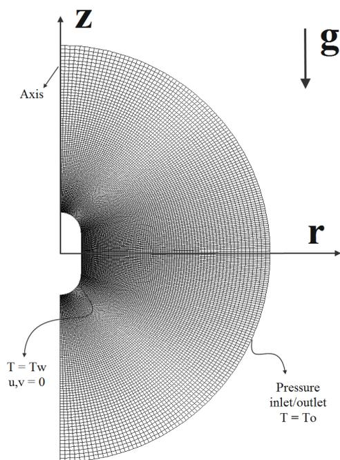
Figure 2. Computational domain and boundary conditions
