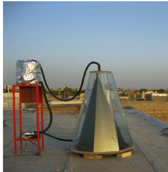
Fig. 3 The conical solar collector used in this study
