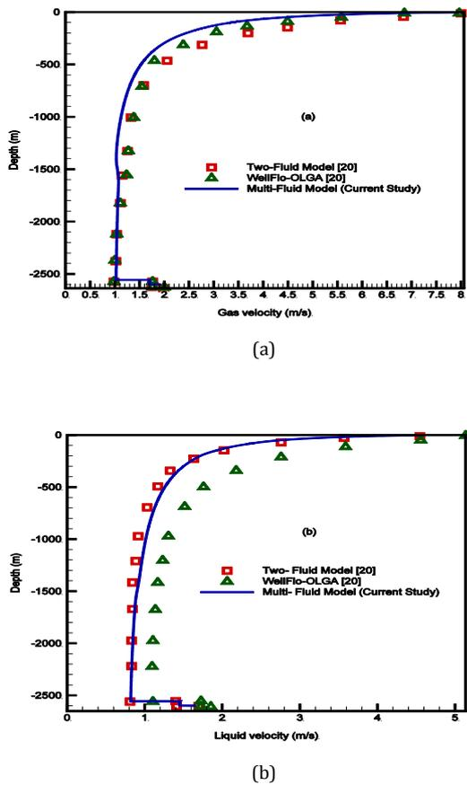
Figure 2. Variation of (a) gas -(b) liquid velocity along the Muspac-53 annulus.
