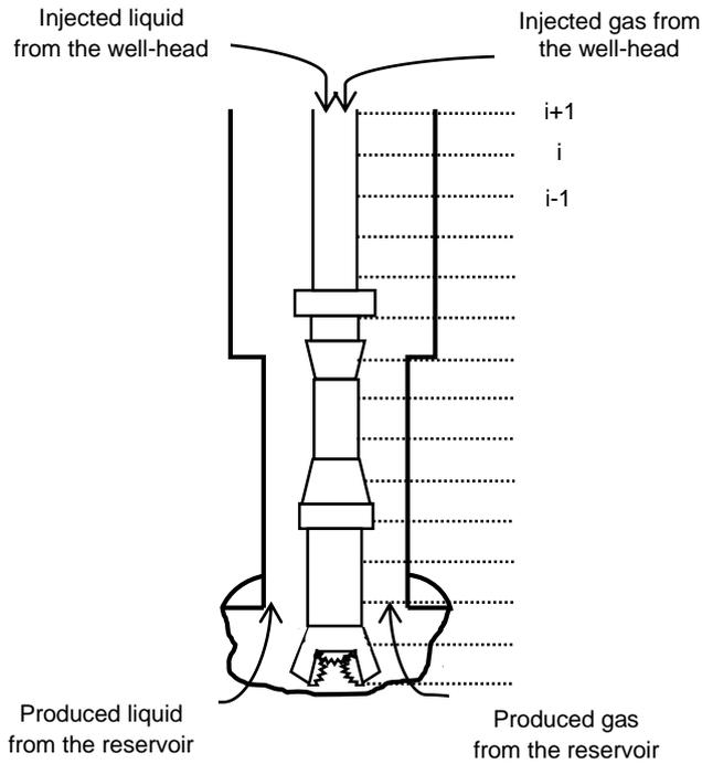
**Figure 1.** Fluid flow in the annular space during UBD operations.
