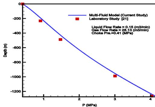
Figure 3. Comparison of pressure variation with Lage and Time laboratory study [22].
