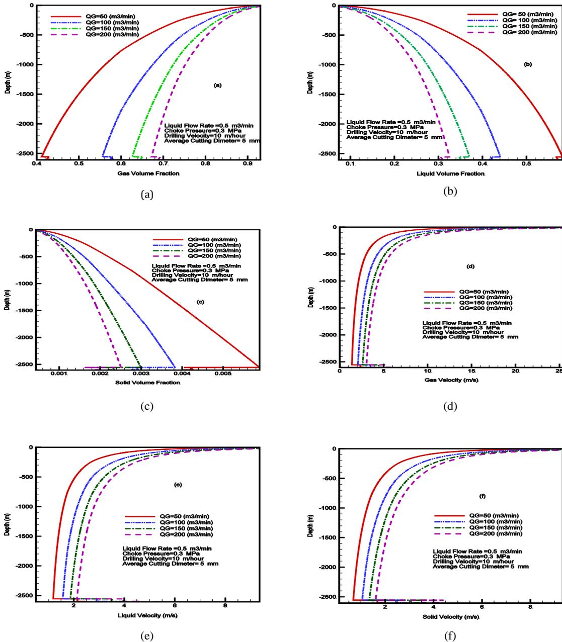
Figure 4. The effects of injected gas flow rate on the annulus flow characteristics.
