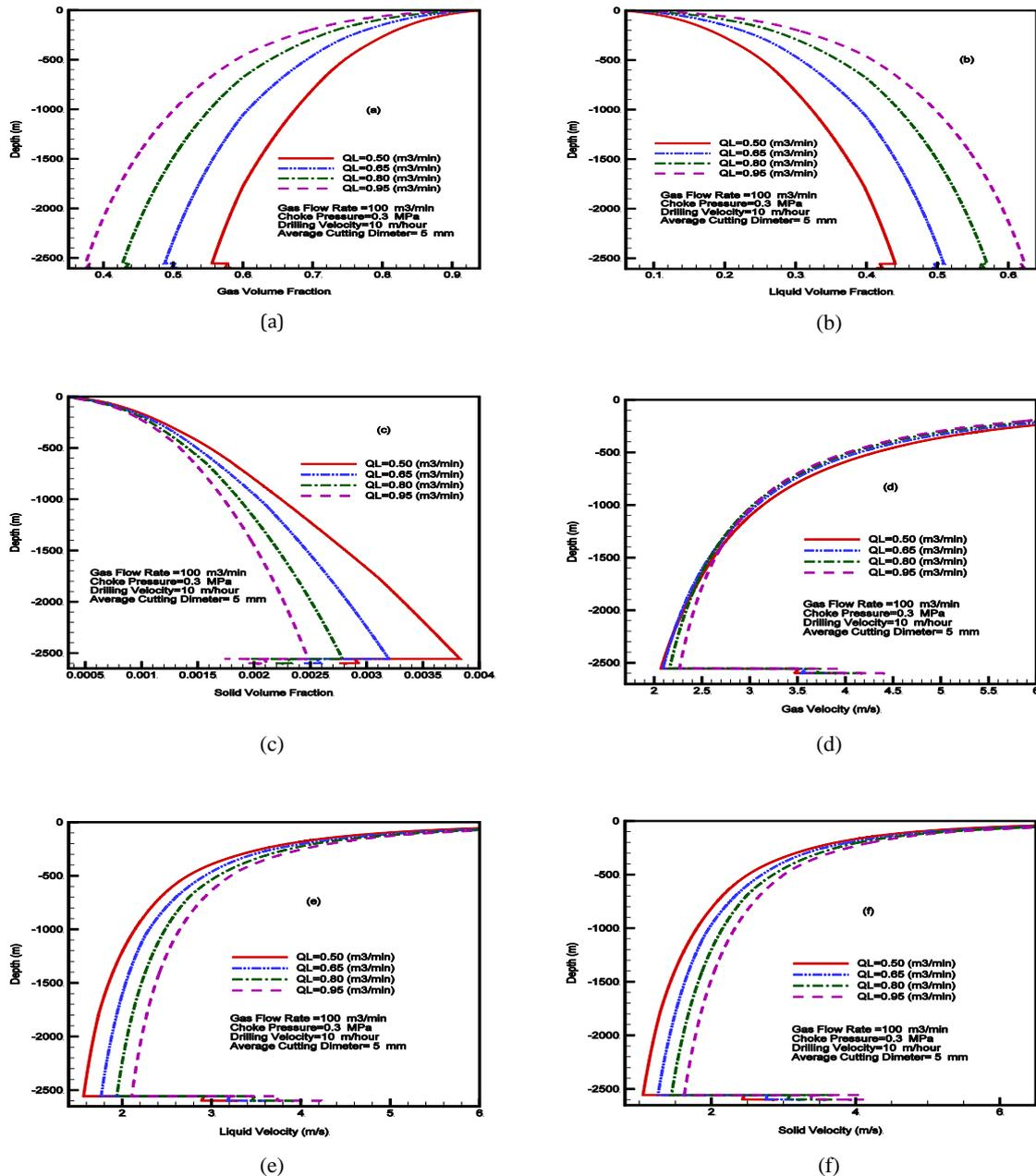
Figure 5. The effects of injected liquid flow rate on the annulus flow characteristics.
