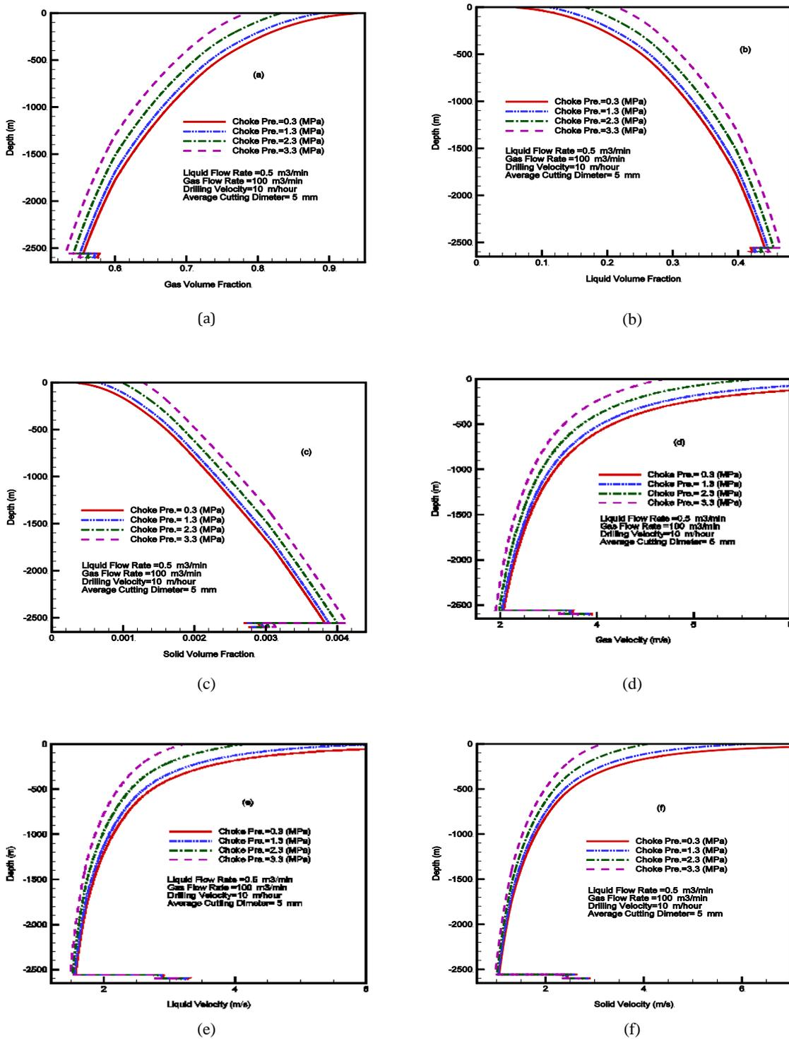
Figure 6. The effects of choke pressure on the annulus flow characteristics.
