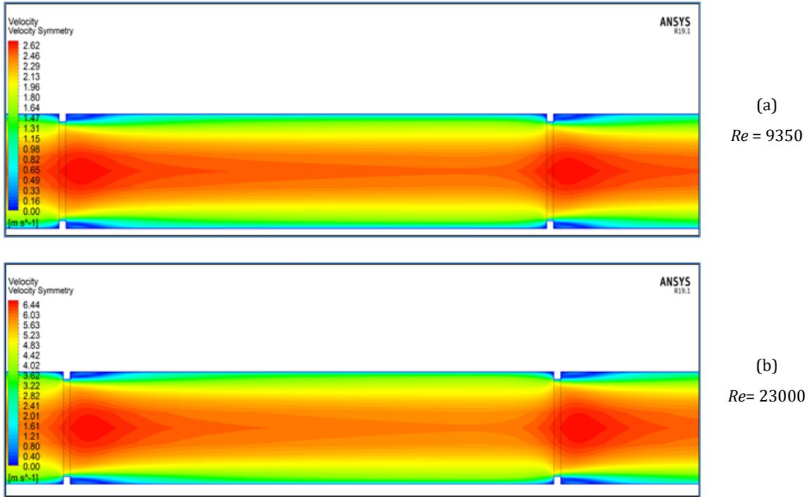
Fig. 5. Velocity contours at 1% nano-fluid concentration for (a)  $Re = 9350$  (b)  $Re = 23000$
