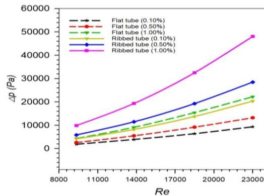
Fig. 9. Variation of pressure drop with Reynolds number
