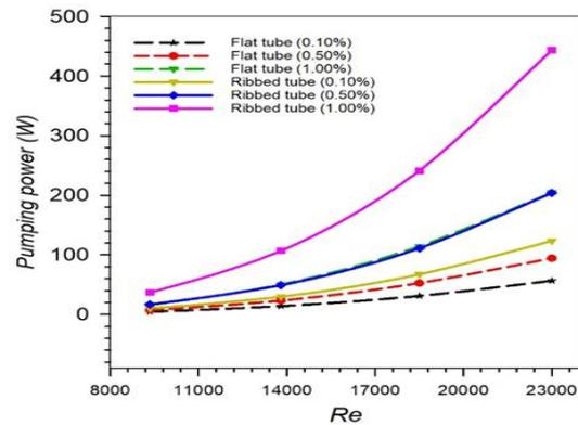
Fig. 10. Variation of pumping power with Reynolds number
