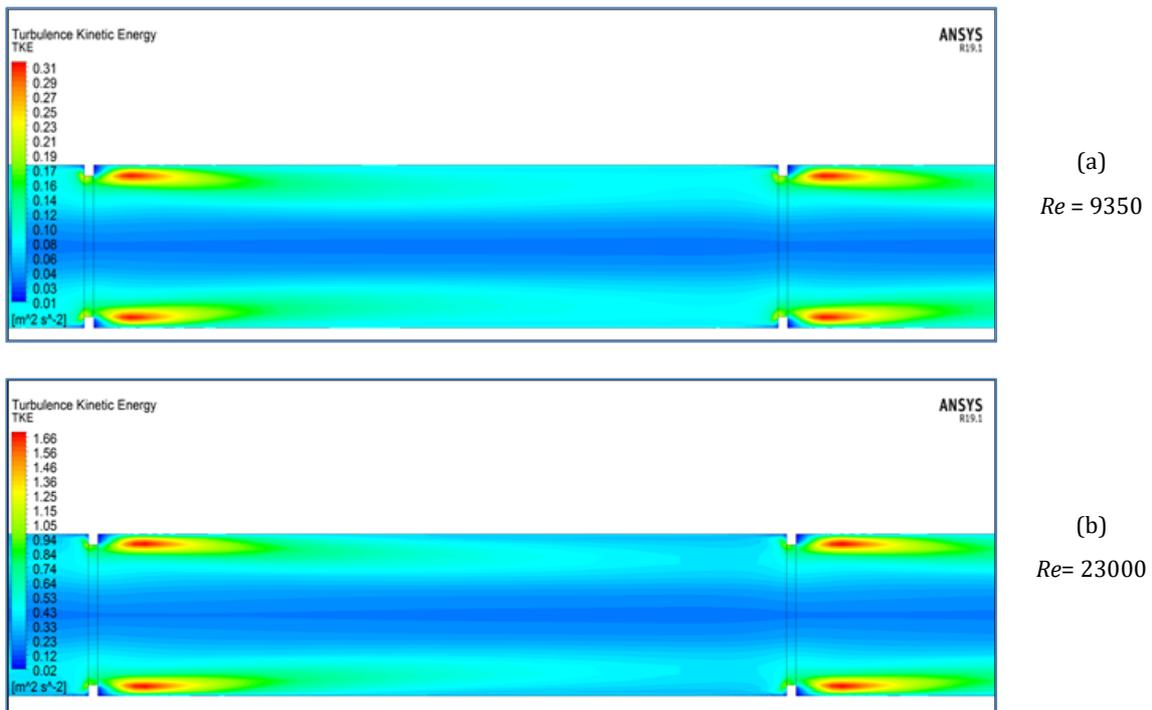
Fig. 6. Turbulent Kinetic Energy contours at 1% nano-fluid concentration for (a)  $Re = 9350$  (b)  $Re = 23000$
