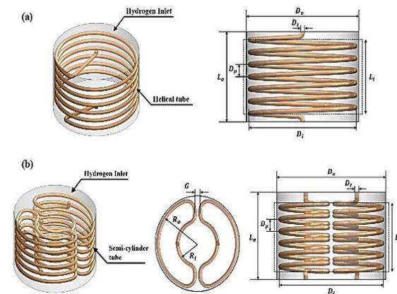
Figure 16. Characteristics of selected geometries for metal hydride reactors. (a) With a helical tube heat exchanger and (b) a semi-cylindrical tube heat exchanger
