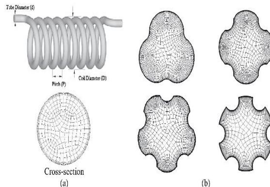
**Figure 13.** (a) Helical coil design and mesh generation. (b) Helical cross-sections with lobes
