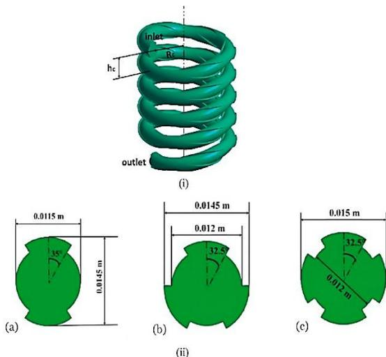
**Figure 11.** (i) A helix coil schematic (ii) Scheme of a head-ribbed coil
