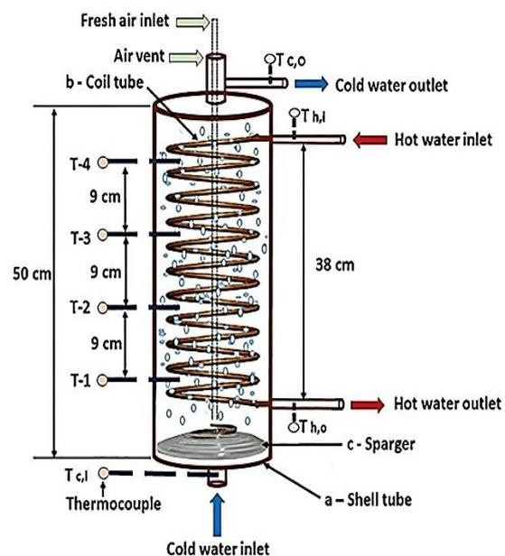
Figure 3. Vertical coiled heat exchanger with bubble generator
