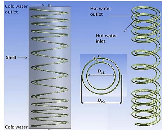
Figure 15. Schematic of shell and double coil tube
