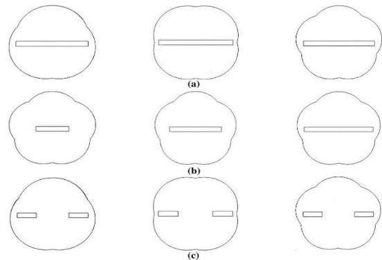
**Figure 12.** 2D schematic of the different studied geometries of the cross-section of coil tube equipped with different types of twisted tape
