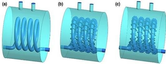
**Figure 10.** Display of the present study geometry in (a) simple, (b) circular finned, and (c) cut circular finned heat exchangers.
