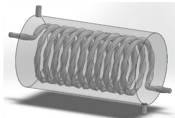
Figure 9. Display of shell and helically corrugated coiled tube heat exchanger
