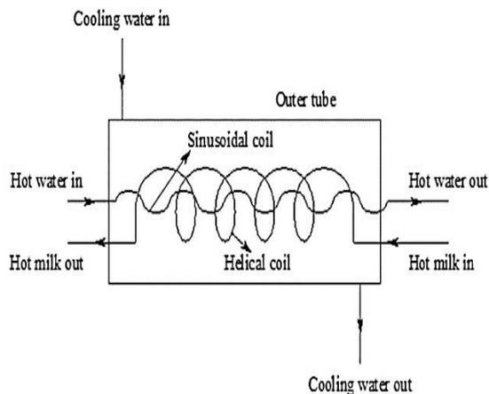
Figure 6. Triple-fluid heat exchanger schematic
