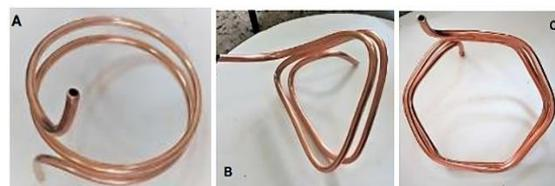
Figure 17. (A) Helical coil, (B) Triangular coil, and (C) Hexagonal coil
