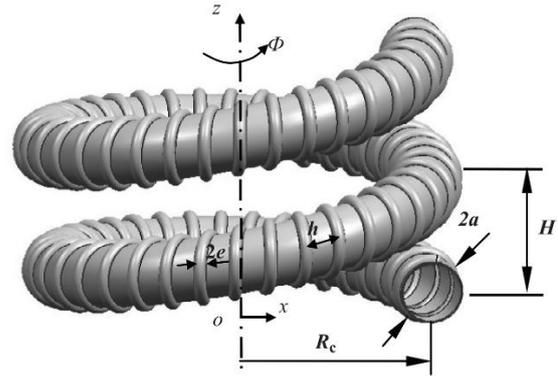
Figure 7. Spiral-corrugated helical tube
