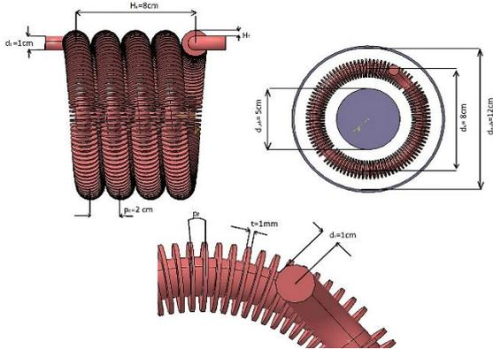
Figure 14. The heat exchanger's geometry
