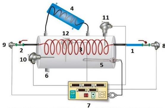
1. Inlet hot water, 2. Outlet hot water, 3. Helical tube, 4. Condenser, 5. Heater (2000 W), 6. Evacuation duct, 7. Thermocouple display box, 8. Inlet cold water thermocouple, 9. Outlet cold water thermocouple, 10, 11, 12. Water bath thermocouple
