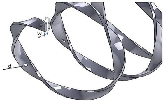
Figure 8. Perforated twisted tape
