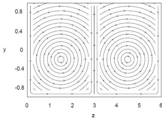
**Fig. 9.** Vector plot of perturbation velocities of plane Couette flow for  $Re = 5000$  and  $S = 0.0015$  at  $x = 3\lambda/4$  with  $S$  being the transpiration amplitude and  $\lambda$  being the wavelength of wall transpiration (Floryan [113]).
