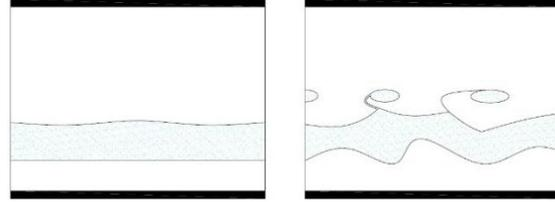
**Fig. 7.** Visualization of (a) a pair of streamwise vortices before the transition and (b) hairpin vortices after the transition in a channel. Note that the direction of the flow is from the left to the right, and the upper and lower boundaries are the channel walls (Philip et al. [101]).
