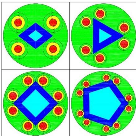
**Fig. 3.** Space-averaged velocity vectors and contours of axial velocities illustrate the streamwise vortices and locations of streamwise streaks at the cross-section of a pipe, respectively. High-speed axial streaks are near the walls, and low-speed ones are near the centers (Faisst and Eckhardt [39]).
