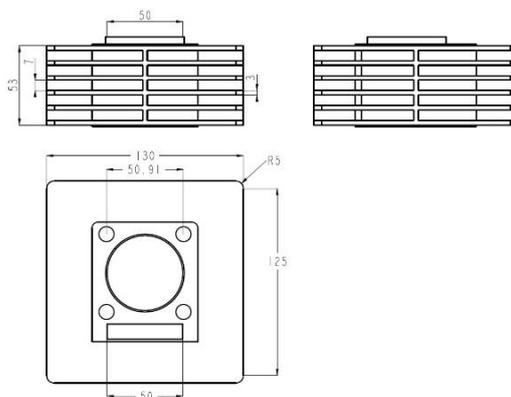
Fig. 1. Rectangular-shaped engine fin body
