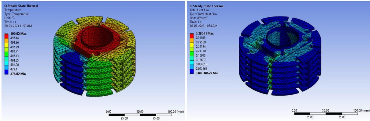
Fig. 12. Circular-shaped engine fin body with slot a) Temperature variation; b) Heat flux variation
