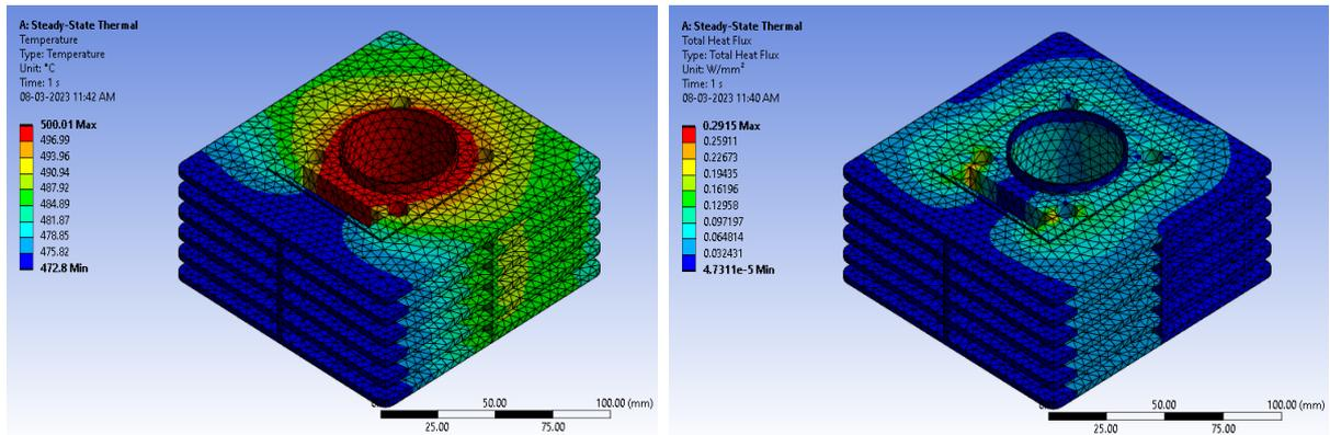
Fig. 9. Rectangular-shaped engine fin body a) Temperature variation; b) Heat flux variation
