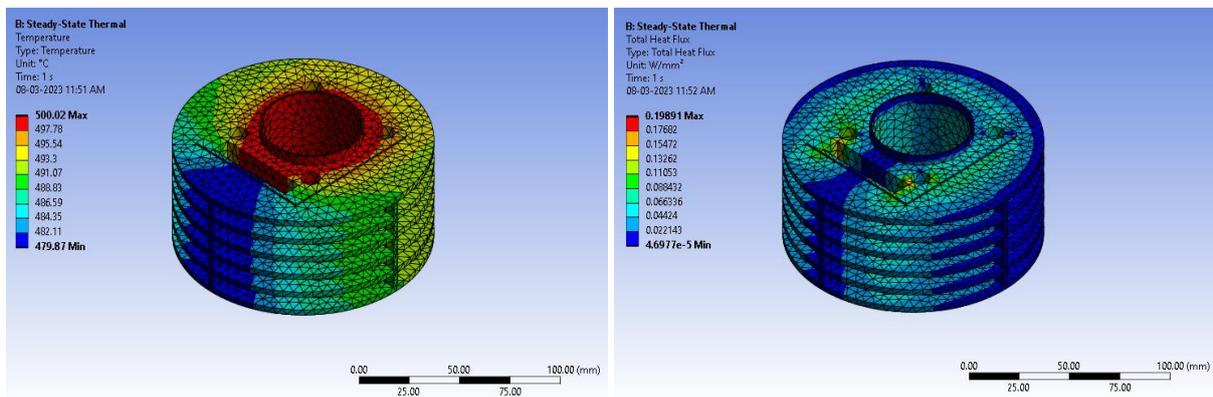
Fig. 11. Circular-shaped engine fin body a) Temperature variation; b) Heat flux variation
