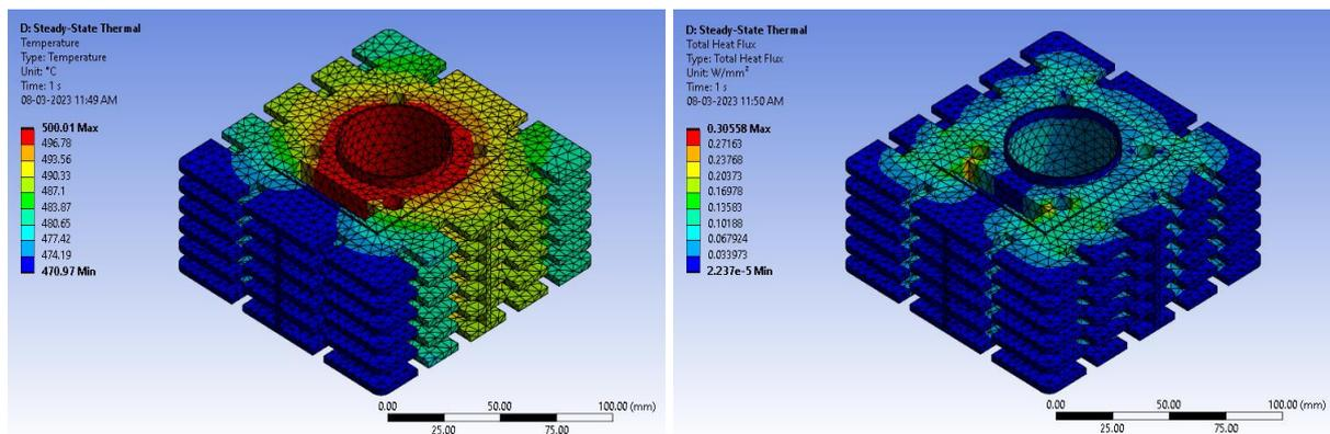
Fig. 10. Rectangular-shaped engine fin body with slot a) Temperature variation; b) Heat flux variation
