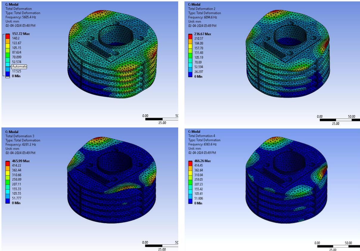
Fig. 7. Cylindrical-shaped engine body –mode shapes 1, 2, 3,4
