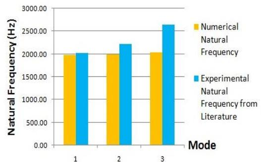
Fig. 8. Simulation model versus Experimental validation based on natural frequency
