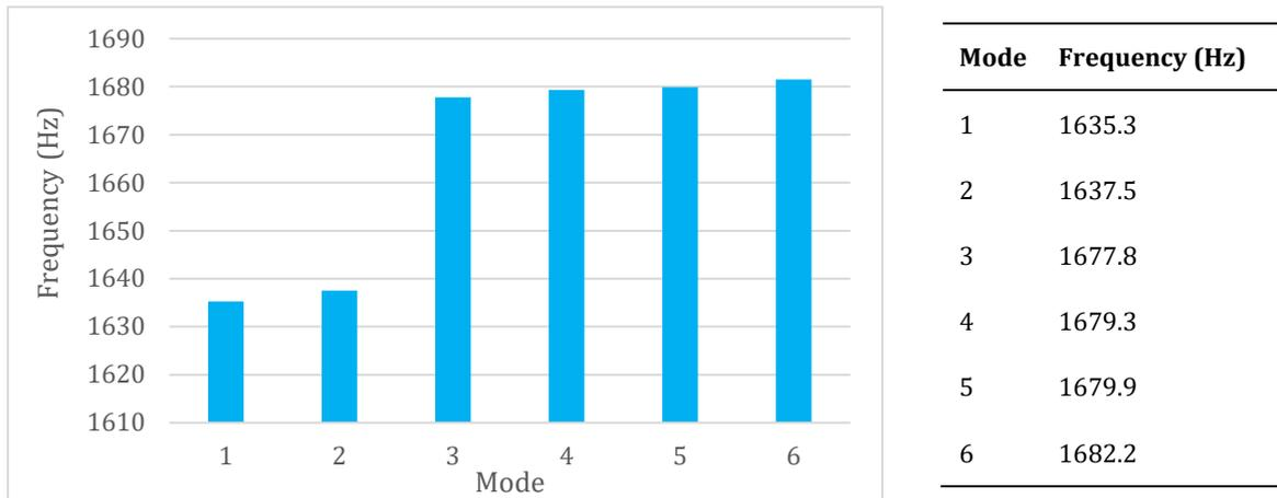
Fig. 15. Natural frequency plot for Rectangular slotted fin
