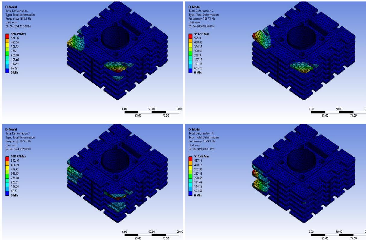
Fig. 14. Rectangular shape engine body (slotted) Mode shapes 1, 2, 3, 4
