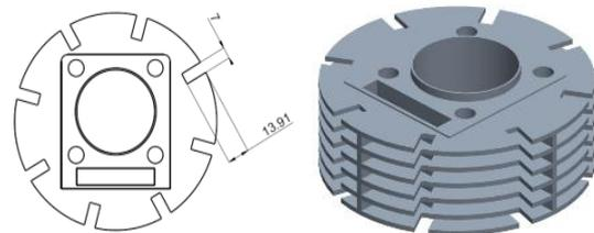
Fig. 4. Circular-shaped engine fin body with slot
