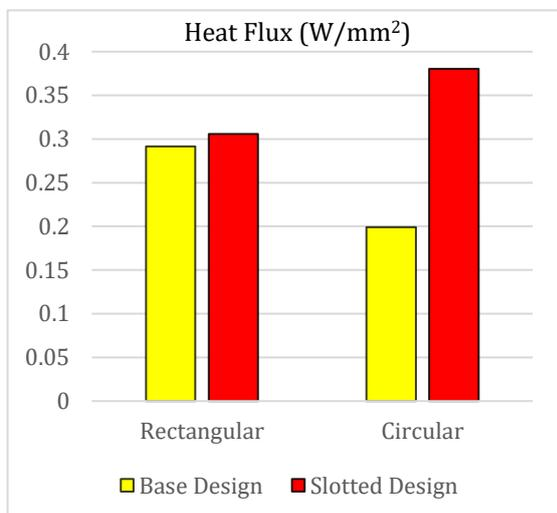
Fig. 18. Comparison of Heat flux of different profile
