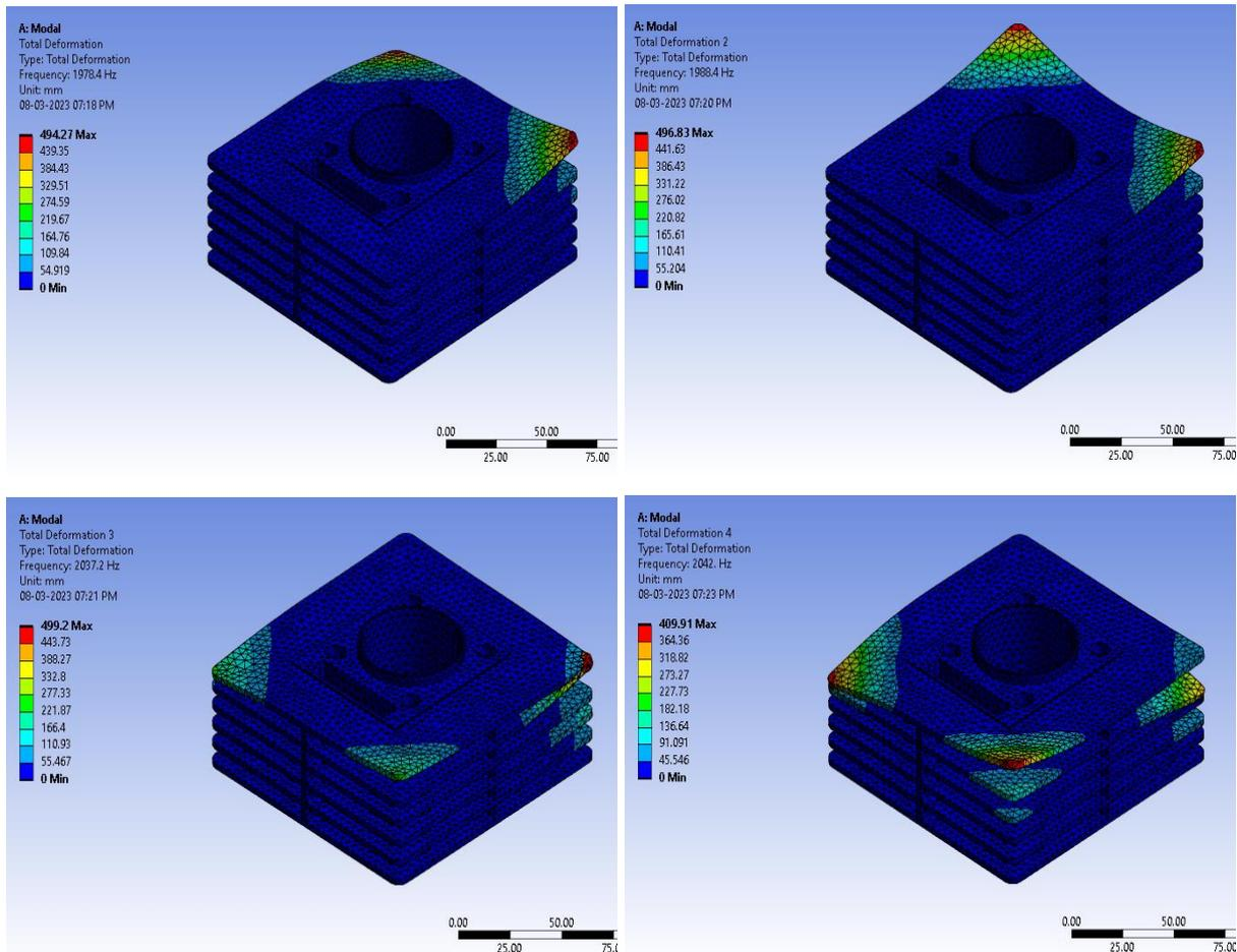
Fig. 6. Rectangular-shaped engine fin body –Mode Shapes 1, 2, 3, 4
