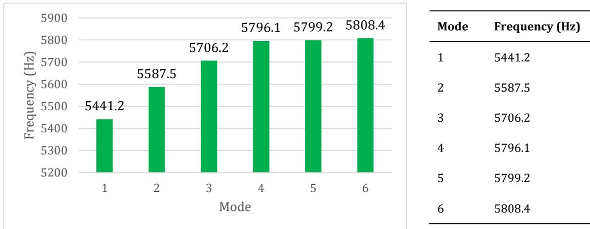
Fig. 17. Natural frequency plot for Cylindrical slotted fin
