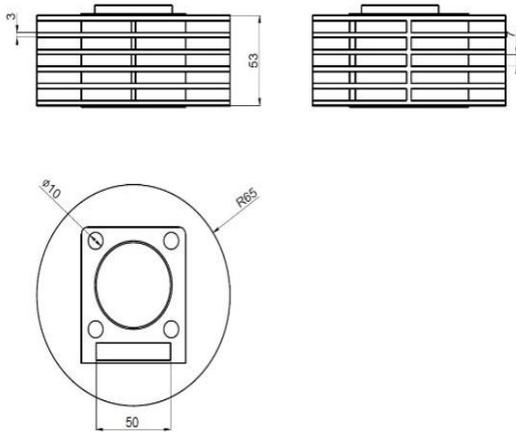
Fig. 2. Circular-shaped engine fin body
