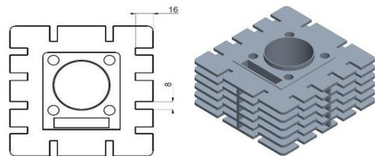
Fig. 3. Rectangular-shaped engine fin body with slot
