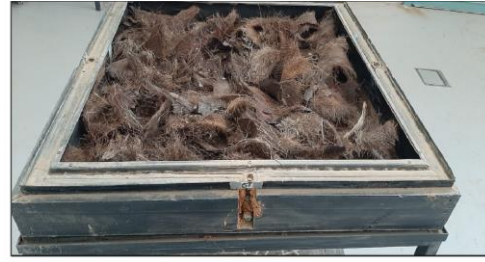
Fig. 1. Application of palmately leaf as the natural fiber in solar still's basin proposed by Alshqirate et al. [48]
