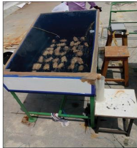
Fig. 7. Application of Ridge gourd material in solar still's basin proposed by Suraparaju et al. [66-70]
