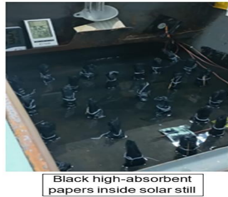
Fig. 3. Application of cellulose-based absorbent material in solar still's basin proposed by Mandev et al. [56]
