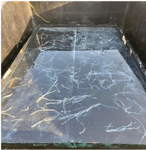
Fig. 5. Application of agar-agar fiber in solar still's basin proposed by Sampathkumar and Natarajan [63, 64]
