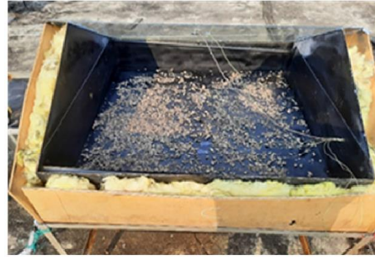
Fig. 6. Application of oil palm shells material in solar still proposed by Sibagariang et al. [65]
