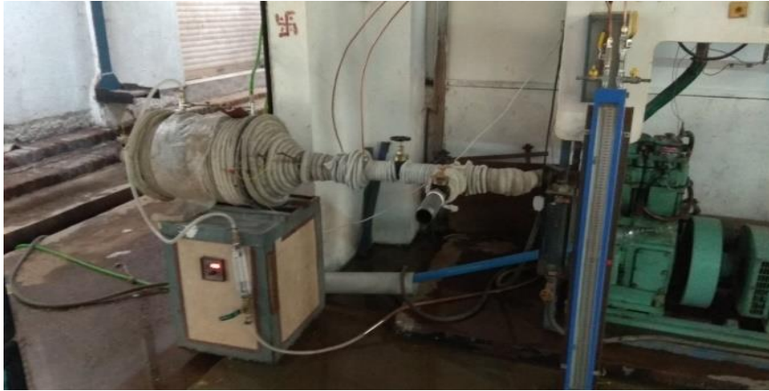
Fig. 5. Shell and helical cone coil heat exchanger setup
