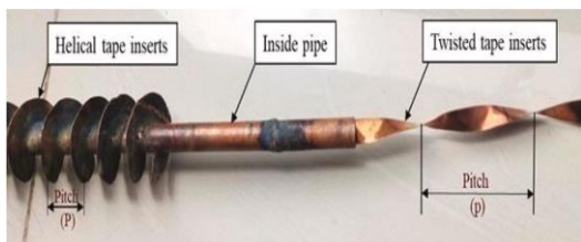
Fig.10a A photograph of twisted tape inserted in tube with helical tapes over tube.[52]
