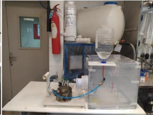
Hot vapor set up with fan
