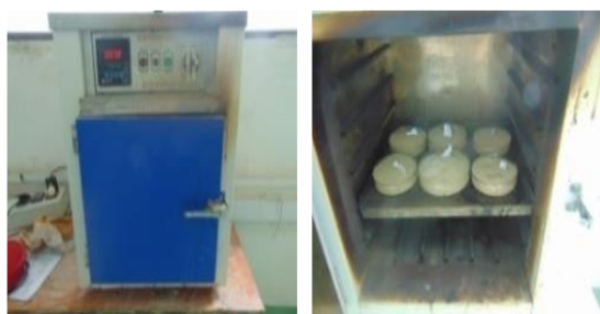
Fig. 2. Teff grain in the oven for moisture content measurement
